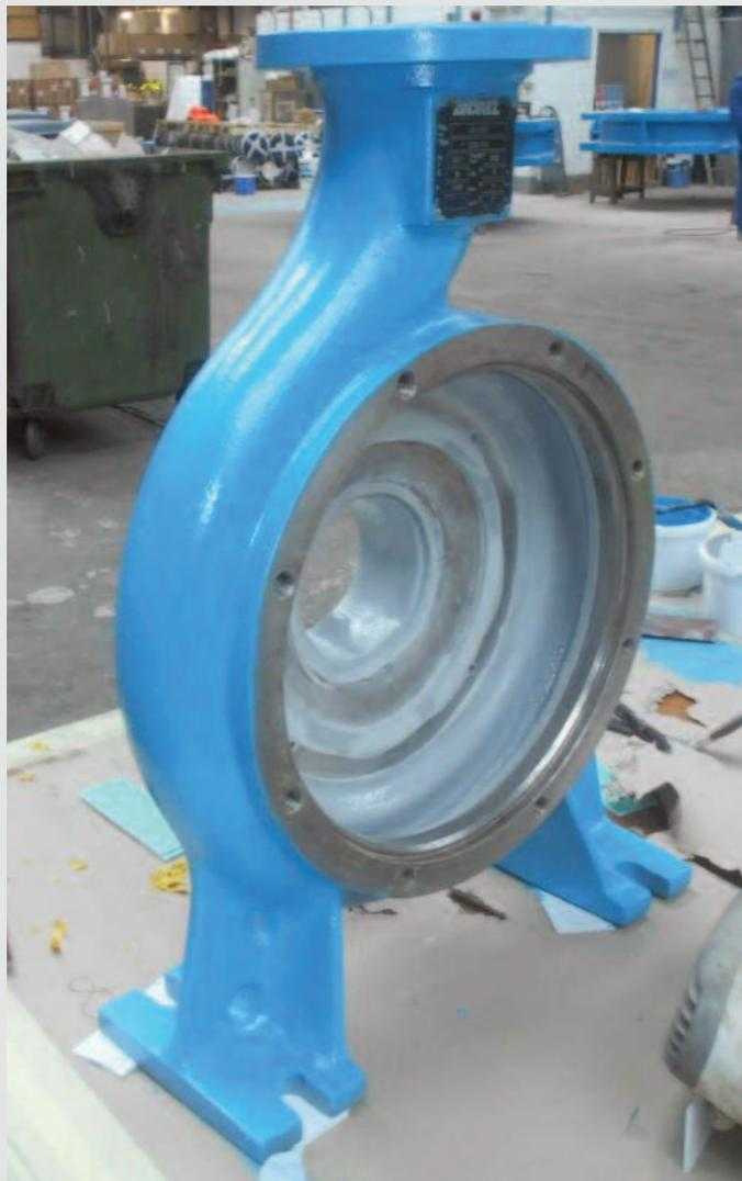
Volute pump casing on arrival at works and following refurbishment and coating with abrasion resistant Plasmert HTE.
