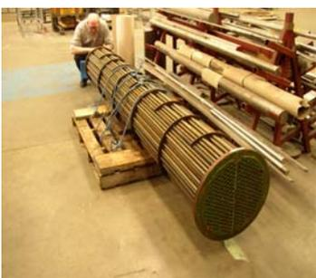
Corrocoat offers a specialist service for tube bundles, including fitting ‘Corrosert’ tube nest inserts to protect against further corrosion.
