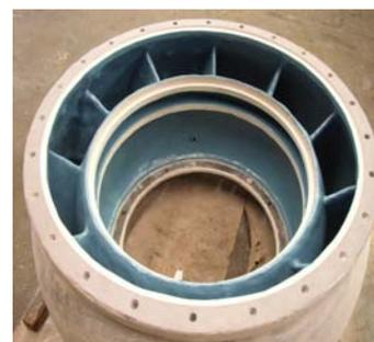
*Pump bowl after repairs have been completed*
