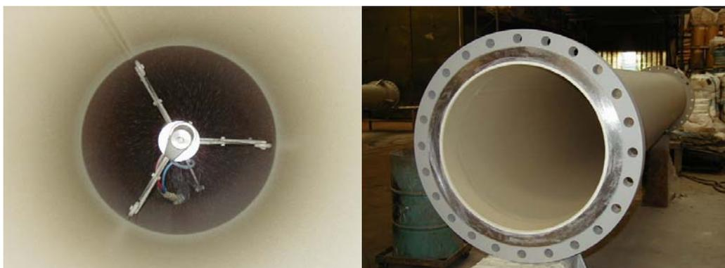
*Coating pipe internals using Corrocoat's proprietary internal pipe spraying rig*
