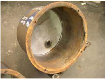
*Brake cylinder prior to coating*
