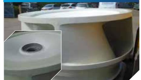
The impeller was then sent back to the Corrocoat workshop to be coated with Corroglass 600.
