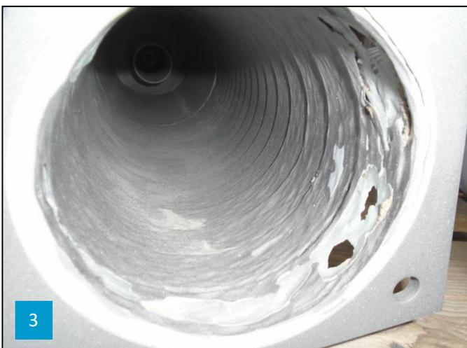
**1: On arrival at workshops. 2: Through wall abrasion damage. 3: Internal view of abrasion damage post abrasive blasting.**
